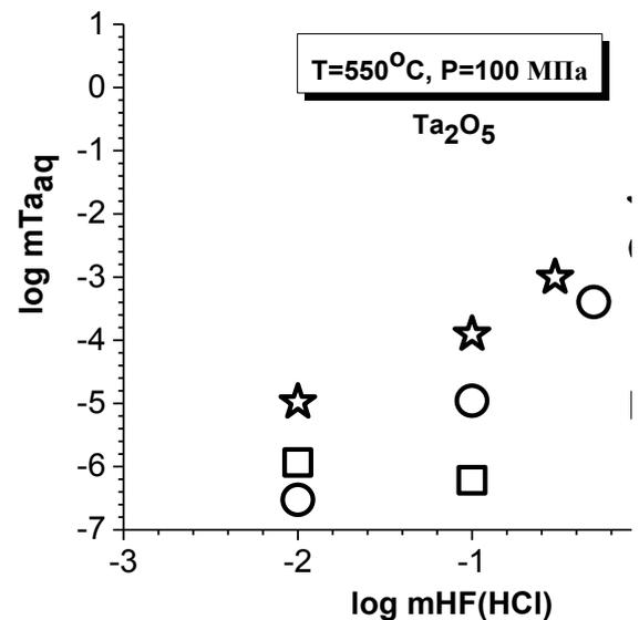
**Fig.1.** The concentration dependence of  $Ta_2O_5$  solubility in mixed solutions of (HF + HCl) at  $T = 550$  °C and  $P = 100$  MPa (Co-CoO buffer)
