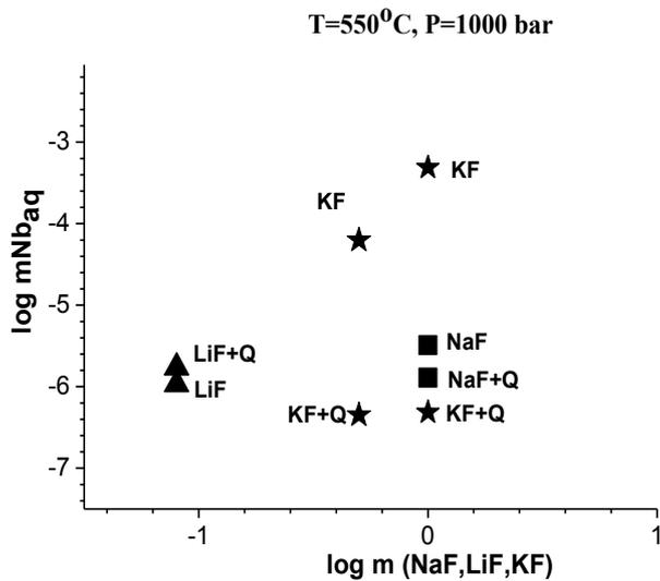
**Fig. 4.** Pyrochlore solubility in the solutions 0.08M LiF; 1M NaF; 0.5 and 1M KF at  $550^{\circ}\text{C}$  and  $P = 1$  kbar (in the presence of quartz and without it).
