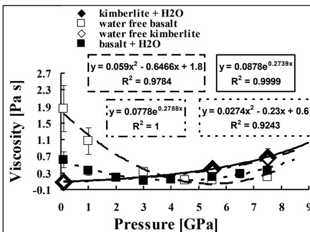
Fig. 3. Isothermal (1800 °C) dependence of the viscosity of water free and water bearing kimberlite and basaltic melts on pressure (uncertainties of experimental and calculating data are  $\pm 30\%$  rel.).
