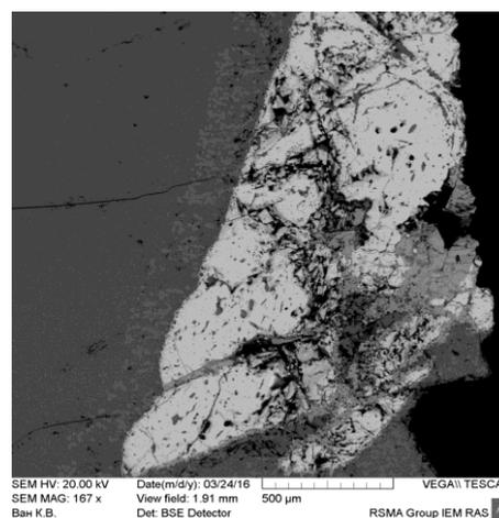
**Fig. 7.** SEM-photography. Light-pyrochlore, dark-silicate glass (850°C, 1kbar).
