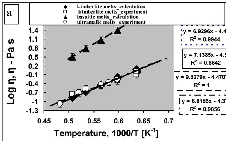
Fig. 1. Temperature dependence of the viscosity of water free ultramafic, kimberlite and basaltic melts (uncertainties of experimental and calculating data are  $\pm 30\%$  rel.). a - Pressure is 100 MPa, b - Pressure is 5.5 GPa,
