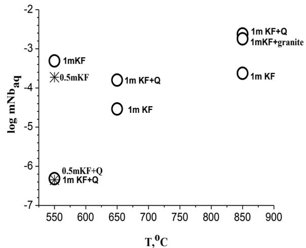
**Fig. 5.** Pyrochlore solubility in the solutions 0.5 and 1M KF at  $550^{\circ}$ ,  $650^{\circ}$  and  $850^{\circ}\text{C}$  and  $P = 1$  kbar (in the presence of quartz and without it).
