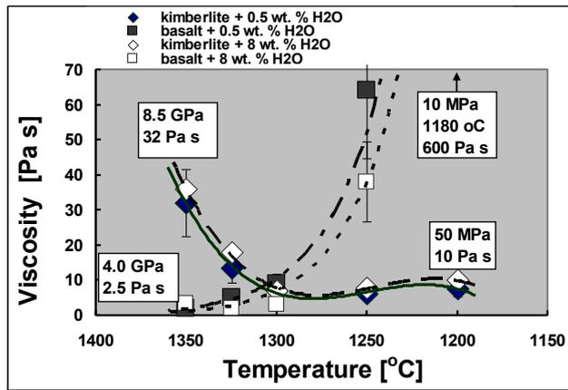
Fig. 4. Changing of the viscosity of water free and water bearing kimberlite and basaltic magmas during their origin, ascent from Earth’s mantle to the crust and during volcanic eruptions.
