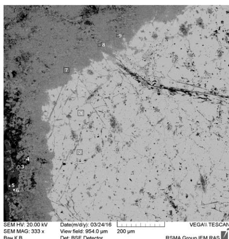
**Fig. 6.** SEM-photography. Light –pyrochlore, dark- silicate glass (650°C, 1kbar).
