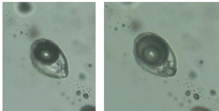
**Fig. 2.** Layering of liquid into two phases at heating of the inclusion. On the left is room temperature, on the right is 352°C
