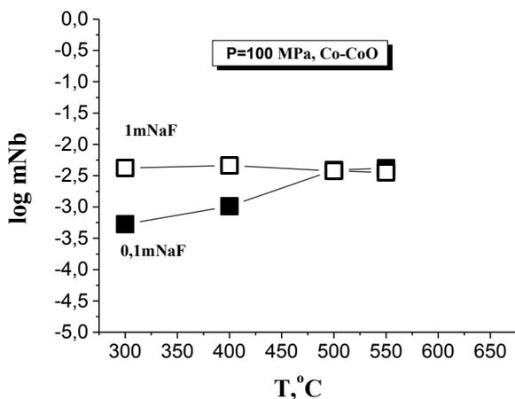
Fig.1. The temperature dependence of Nb<sub>2</sub>O<sub>5</sub> solubility in NaF solutions at P = 100 MPa (Co-CoO buffer)
