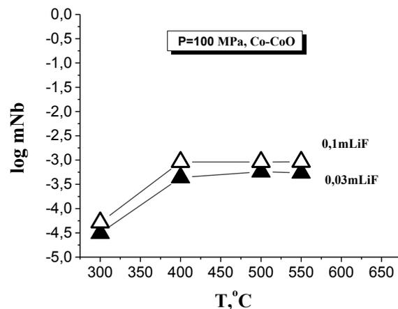
Fig.2. The temperature dependence of Nb<sub>2</sub>O<sub>5</sub> solubility in LiF solutions at P = 100 MPa (Co-CoO buffer)
