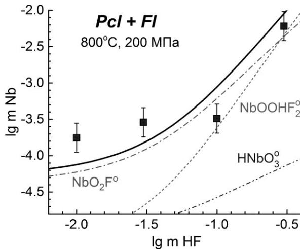
**Fig. 2.** Effect of  $m \text{ NaF}$  on Nb content in solutions that are in equilibrium with Pcl and Fl at  $800^\circ \text{C}$  and  $P = 200 \text{ MPa}$  (experimental and calculated data). The lines show the trend change of  $m \text{ Nb}$  on  $m \text{ HF}$  and the concentration of the predominant species of  $\text{Nb}^{5+}$ .
