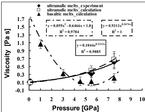
Fig. 2. Isothermal (1800 °C) dependence of the viscosity of ultramafic and basaltic melts on pressure (uncertainties of experimental and calculating data are  $\pm 30\%$  rel.).
