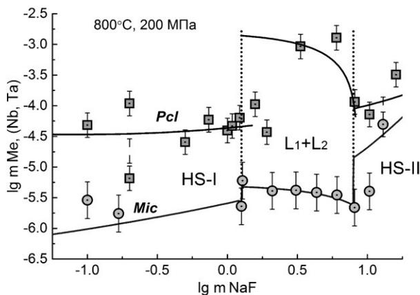
**Fig. 3.** Effect of  $m \text{ NaF}$  on Nb content and Ta in solutions that are in equilibrium with Pcl and Fl at  $800^\circ \text{C}$  and  $P = 200 \text{ MPa}$ . The lines show the trends change of  $m \text{ Nb}$  and  $m \text{ Ta}$  on  $m \text{ NaF}$ .
