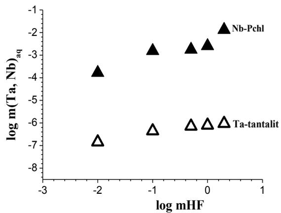
**Fig. 3.** Concentration dependence of Nb and Ta content in (HF + HCl) fluids when Nb<sub>2</sub>O<sub>5</sub> and Ta<sub>2</sub>O<sub>5</sub> are dissolved (T = 550 ° C, P = 1000 bar, Co-CoO buffer)
