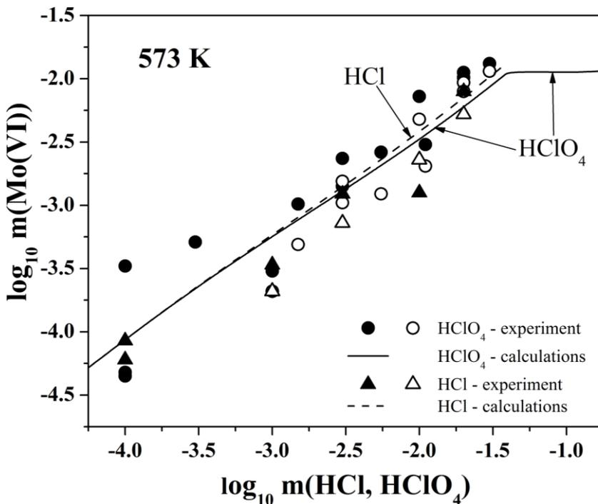
**Fig. 1. Experimental (symbols) and calculated (lines) values of solubility of  $\text{CaMoO}_4$  in solutions of acids.** The filled symbols represent data of the chemical analysis, open symbols – the weight loss data.
