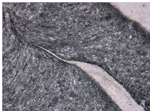
Fig. 4. Microphotography of of an area of zone 1, reflected light. Shear band accommodates a taenite vein (from down right to upper left), the last is thinning and wedging out. Etched in nital. Field of view is 0.22 mm.
