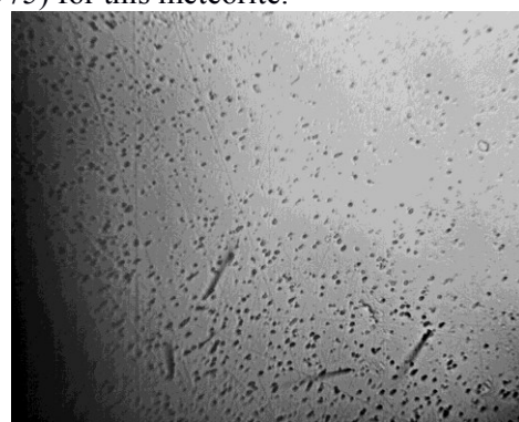
Fig. 4. Fragment of a micrograph of the surface of an olivine crystal (pallasite Marjalahti) with a high gradient of track density. The image size is 284 \times 226 \mu\text{m} .
