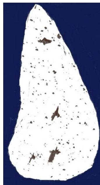
Fig.1. The X-ray tomography data on the distribution of Pt in albite glass.
