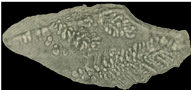
Fig. 1. Crystals of double phosphate in glass of ijolite-urtite composition T 1300°C, composition 4 (see table 1).
