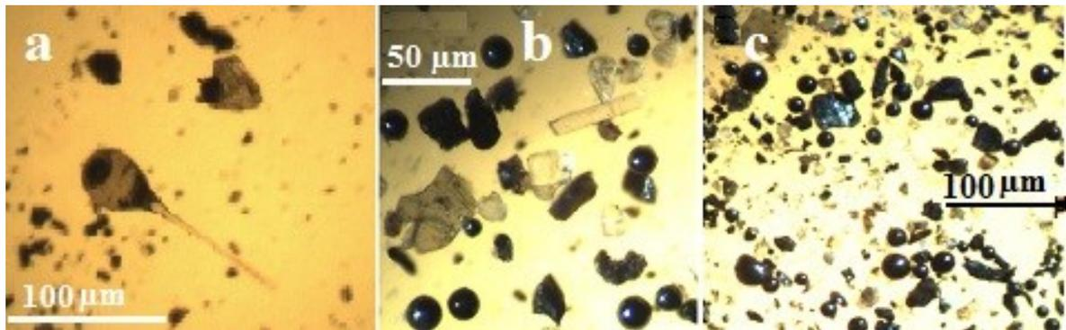
**Fig. 1.** Images (Nikon): **a** – non-magnetic part of the UAD sample; **b, c** – magnetic fraction separated from the sample UAD (with fine mineral admixture).
