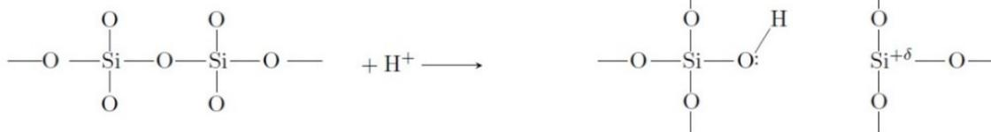
we find that the breaking of 100–200 bonds corresponds to a distance of ~20–40 nm. The proton deceleration time is about  $10^{-13}$  s. In turn, to estimate the number of acts of breaking of Si–O bonds in the near-surface layer of the regolith, we will take the value of 30 nm as the depth of passage of the proton. Then, in this layer with an area of  $1 \text{ cm}^2$  happens
