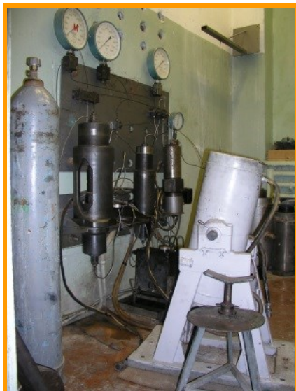
Fig. 1. Internally heated pressure vessel (IHPV).
