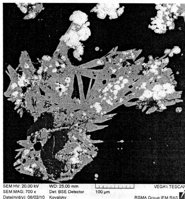
Fig.2 SEM backscattered electron detector image of the polished sample of a two-phase sediment: white - \text{CsBF}_4 , gray - \text{NaCs}(\text{BF}_4)_2 .
